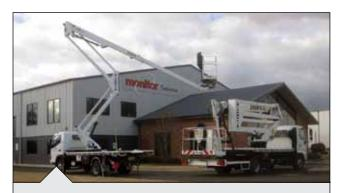
With a choice of stabilizer configurations and S.W.L. options, the PX range can be mounted to very compact and light weight commercial vehicles. In fact, we can even provide a 20 metre boom lift on a car licence!
