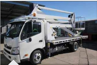
All hoses and wiring are neatly routed inside the PX boom sections, eliminating component damage in harsh applications such as tree maintenance works. The controls are simple, well proven, live hydraulic levers, which provide smooth proportional operation of the booms. A number of operations can be made simultaneously, increasing the speed and accuracy of movement even at full extension.
