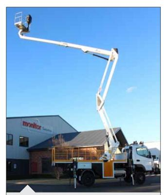
Not only do the PX models excel in horizontal reach, but they also provide a much better vertical lift path which is ideal for working up the face of buildings, signs etc. (209PX pictured on 4x4 Canter.)
